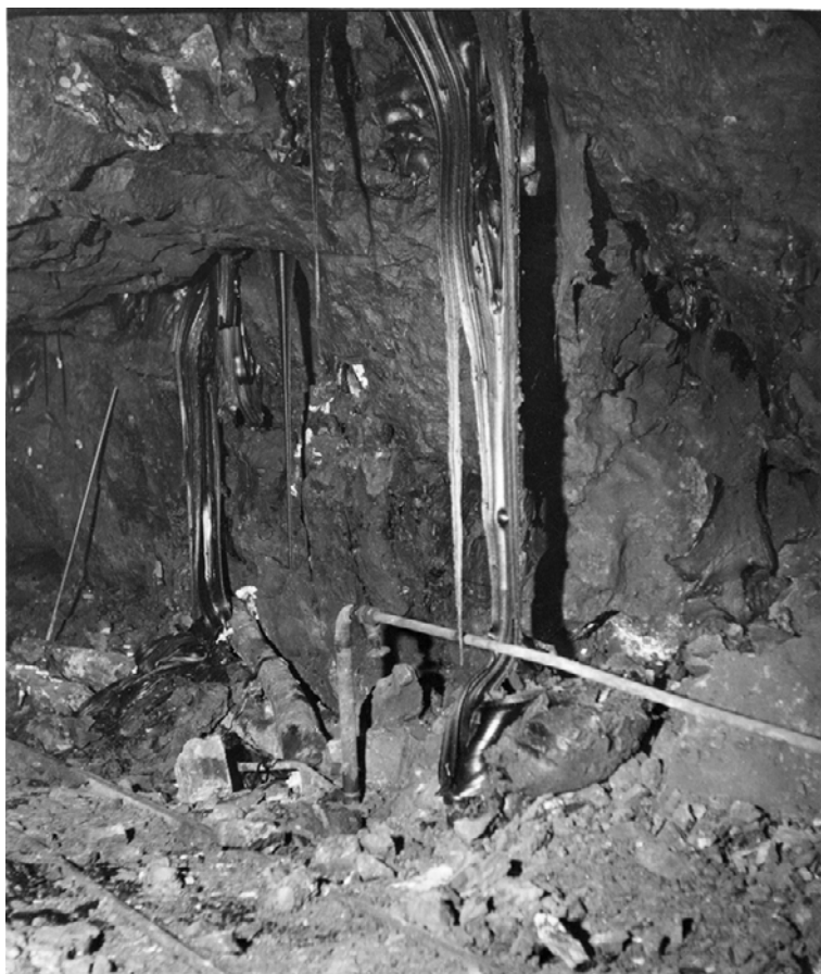
Fig. 2. Viscous bitumen natural flow in a mine tunnel (courtesy of Lettomanoppello City Hall). Estimated 4°–8° API crude oil by visual comparison with fluid samples.
